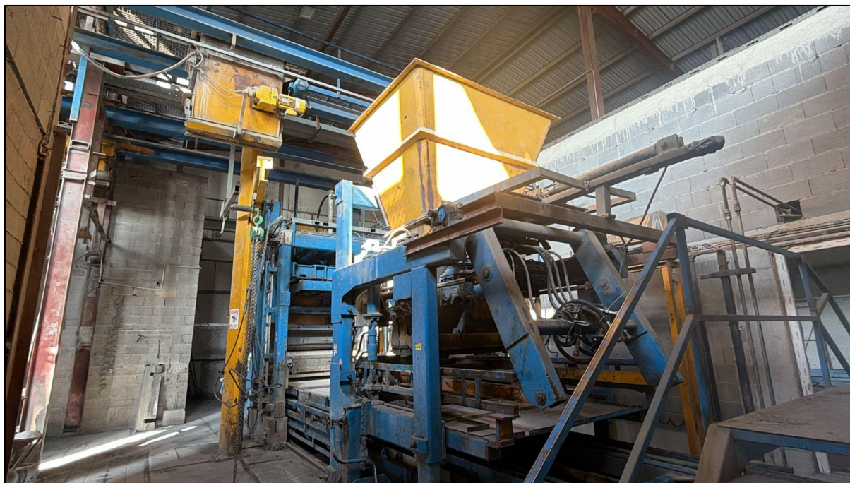
Figure 5. Makina prodhuese me kapacitet 1000-2000 m 2 /h
