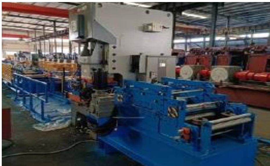
Figura 20. Punching Unit Aluminium Corner.
